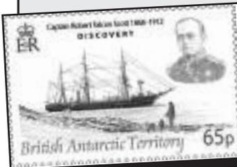
*Discovery, 737 tons 172' x 33' Built 1900 by the Dundee Shipbuilders Company in the yard owned until 1894 by Alexander Stephen & Sons. She was never a whaler/sealer, but built on the well tested lines of such a vessel. She was the last traditional wooden three-masted ship to be built in Britain.*
